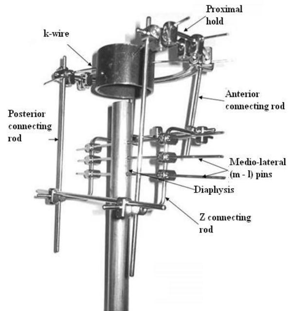
Fig.1 JESS configured on steel tubes
