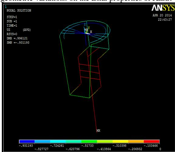
Fig.3 Deformed model of JESS under axial compression
