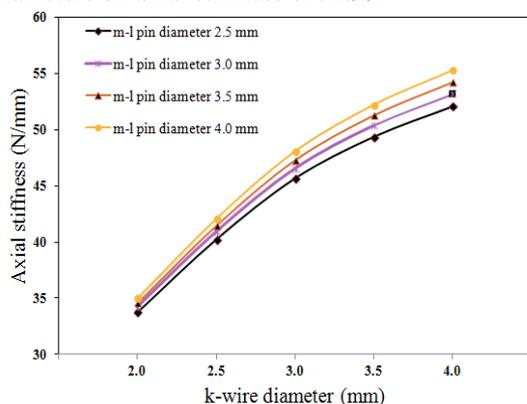
Fig.5 Variation in axial stiffness of JESS for different set of m-l pin sizes
