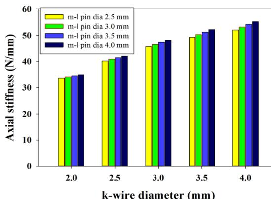
Fig.6 Variation in axial stiffness for varying medio-lateral pin diameter
