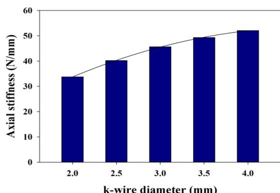
Fig.4 Variation in axial stiffness of JESS with change in k-wire diameter (m-l pins diameter 2.5 mm)
